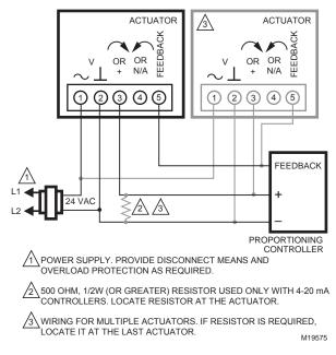
Fig. 13. Wiring for a proportioning controller operating multiple actuators (modulating mode setting).
