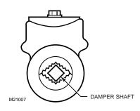
Fig. 3. Proper mounting to square damper shaft.
