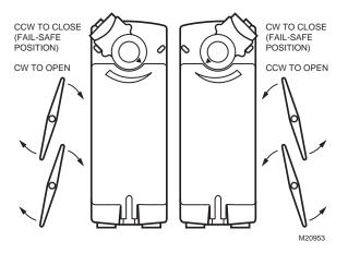
Fig. 2. Spring Return DCA mounting orientation.
