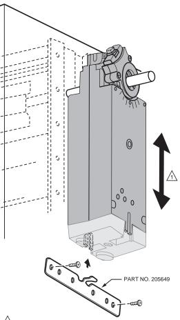
LISUBLE THAT MOUNTING ASSEMBLY PREVENTS ACTUATOR ROTATION AND ALLOWS ACTUATOR TO FLOAT ALONG INDICATED AXIS. WHEN TOO TIGHT, THE RESULTING BINDING CAN DAMAGE THE ACTUATOR OR REDUCE TORQUE OUTPUT. M20956
