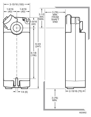
Fig. 1. Dimensional drawing of actuator in in. (mm).
