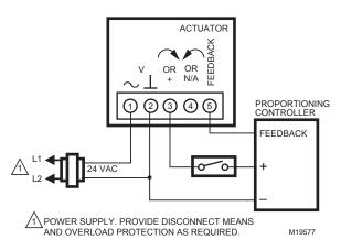
Fig. 15. Override to full close (modulating mode setting).
