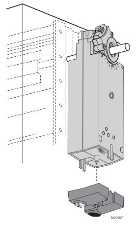
Fig. 8. Removing access cover.
